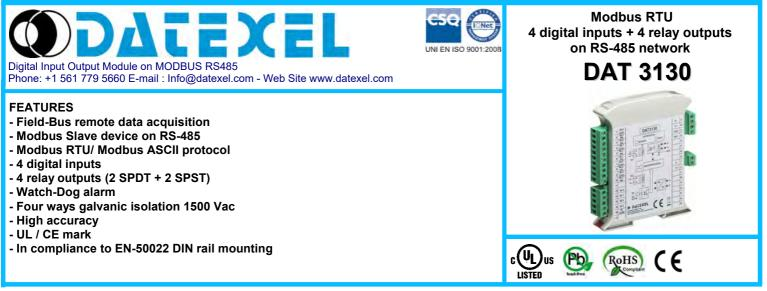
GENERAL DESCRIPTION The device DAT 3130 is able to acquire up to 4 digital inputs and to drive up to 4 relay outputs. The data are transmitted with MODBUS RTU/MODBUS ASCII protocol on the RS-485 network. The device guarantees high accuracy and stable measure versus time and temperature.
