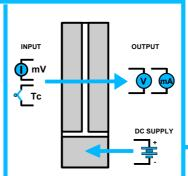
Isolated converter for Tc and mV configurable by Dip-Switch or PC
