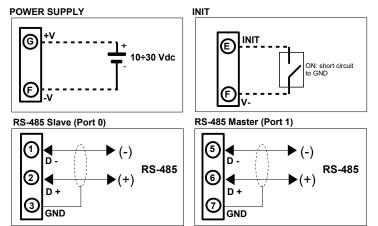
Note: the device must be powered using a power supply unit classified NEC class 2 or SELV with limited energy
