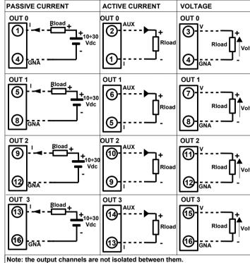
Terminals AUX of channels connected between them. Terminals GNA of channels connected between them
