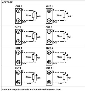
Note: the output channels are not isolated between them. Terminals GNA of channels connected between them.
