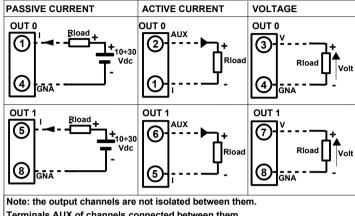
Note: the output channels are not isolated between them Terminals AUX of channels connected between them. Terminals GNA of channels connected between them
