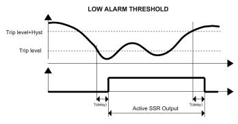
For the low alarm the relay goes on when the input signal is lower than the trip level and after the delay time. The relay goes off only when the input signal is higher than the trip level plus the hysteresis value or when reaches the maximum value of the input scale and after the delay time.
