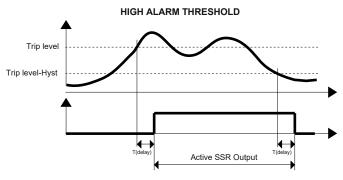
For the **high alarm** the relay goes on when the input signal is higher than the trip level and after the delay time. The relay goes off only when the input signal is lower than the trip level minus the hysteresis value or when reaches the minimum value of the input scale and after the delay time
