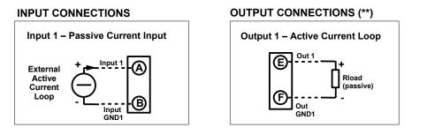
(\*\*) Note: if there is an interruption either in the input or in the output current loop, the output signal will be 0 mA.
