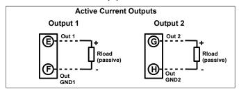
(\*\*) Note: if there is an interruption either in the input or in the output current loop, the output signal will be 0 mA.
