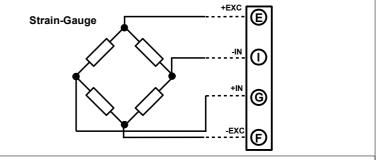
Note: internal connection between terminals I = L and G = H
