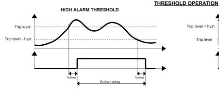
For the high alarm the relay goes on when the input signal is higher than the trip level and after the delay time. The relay goes off only when the input signal is lower than the trip level minus the hysteresis value or when reaches the minimum value of the input scale and after the delay time
