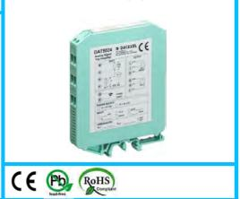
GENERAL DESCRIPTION The economic trip amplifier DAT 5024E is able to accept on its input normalised voltage and current signals coming from both active and passive current loops. Both the trips can be configured as high or low alarm; it is possible to regulate the trip level values by the potentiometers THR1 and THR2 located on the front side of the device. The isolation between input and power supply is 1500 Vac. The isolation between input and the contacts of relays is 1000 Vac.
